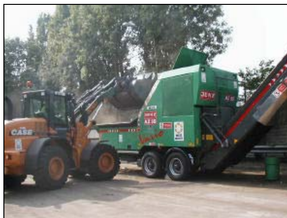
Green waste being loaded into a shredder before being taken by railway to be recycled into compost
